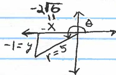
Using the Pythagorean Theorem,  $x^2 + y^2 = r^2 \Rightarrow x^2 + (-1)^2 = (5)^2 \Rightarrow x^2 + 1 = 25 \Rightarrow x^2 = 24 \Rightarrow x = \pm\sqrt{24} \Rightarrow x = \pm 2\sqrt{6}$ . Furthermore, the diagram shows that  $x$  is in the negative direction in  $QIII$ , so  $x = -2\sqrt{6}$ .
